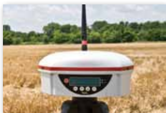
RTK BASE STATION
