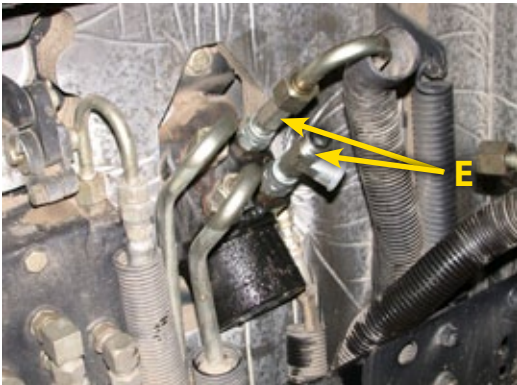
Figure 1-6: Installing the Steering Output Fittings
