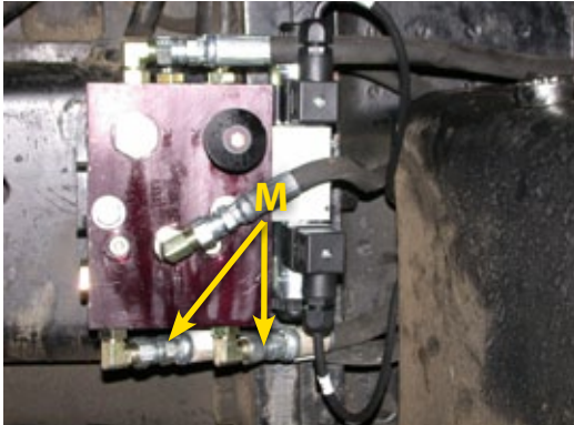
Figure 1-7: Installing the Steering Output Hose
