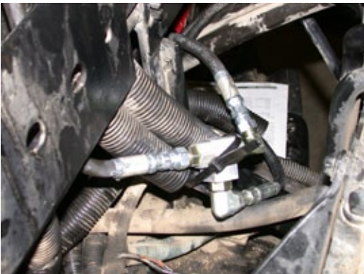
Figure 1-10: Installing the Tractor Load Sense Shuttle/Adapters
